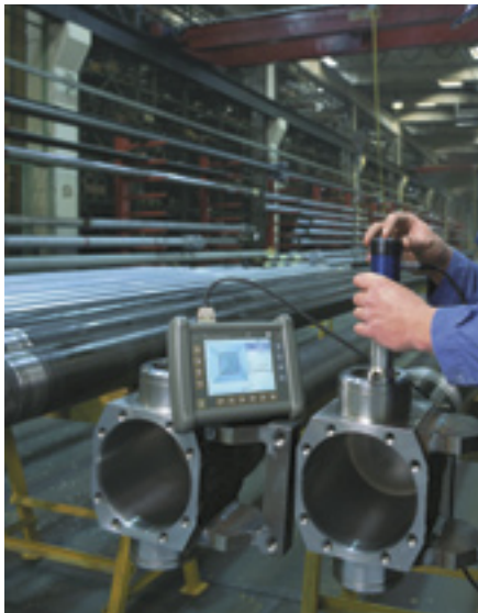
Figure 12: The TIV hardness tester in field use.
