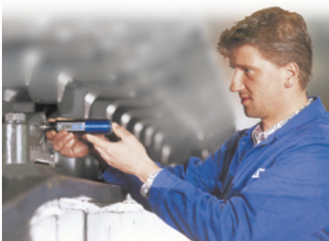
Figure 3: Hardness testing using the DynaPOCKET on the chain of an open-pit mining excavator.
