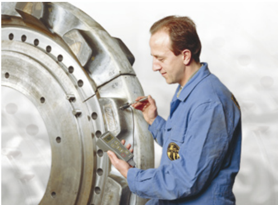
Figure 2: Hardness testing with a rebound hardness tester (DynaMIC) on the drive wheel of a large hydraulic excavator.
