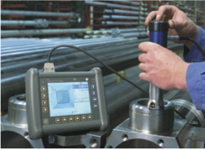
Figure 4: Optical hardness testing using the TIV tester. Checking before final assembly.
