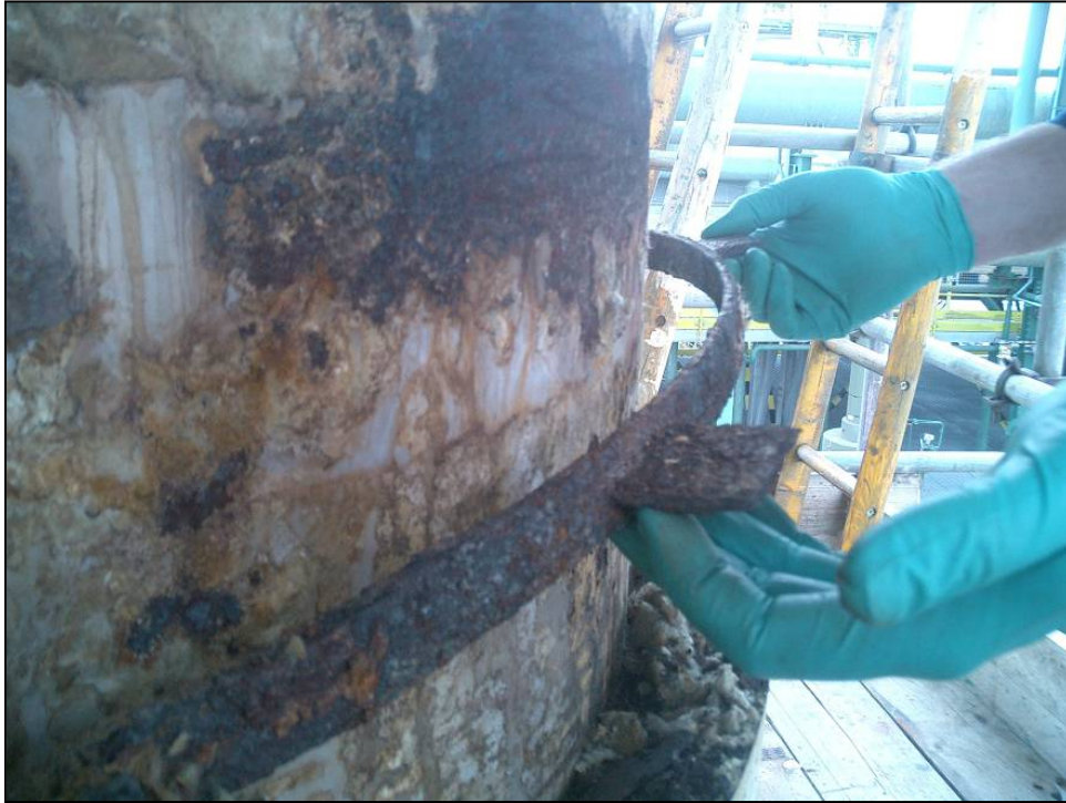
External corrosion on a vertical pipeline. Located at a circumferential insulation clamp.
